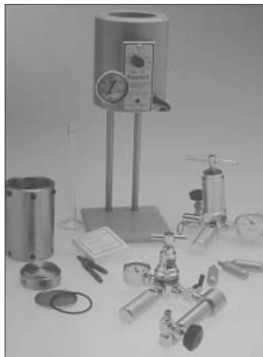
Figure 8: HTHP filter press (API #1 style) (disassembled).
