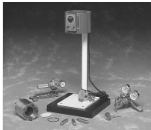
Figure 6: HTHP filter press (disassembled).
