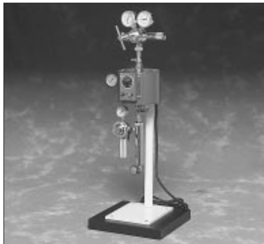
Figure 7: HTHP filter press (MB style - API #II).
